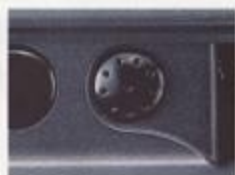
The ASC microphone constantly monitors the noise level.
